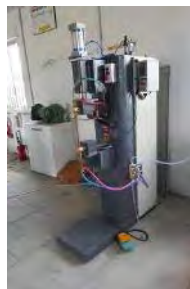
▲ Locally made resistance welder purchased by this institute
