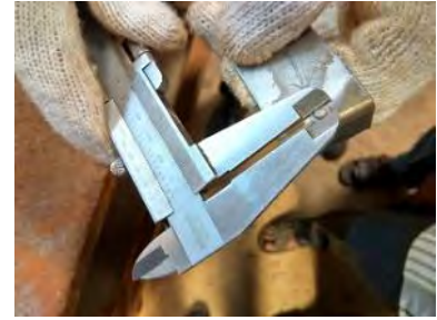
▲ Nugget diameter measurement using calipers
