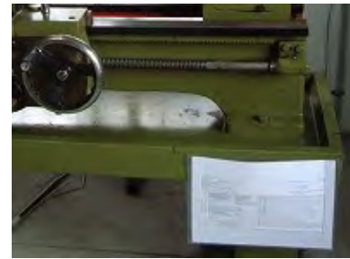
▲ Periodic inspection sheet affixed to a conventional lathe (PCFCT Walajah)
