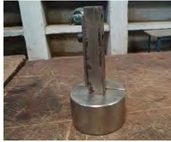
▲ Tool centre height adjustment jig for which guidance was given on manufacture and introduction
