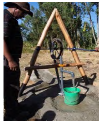
Windlass Model (Wooden body)
