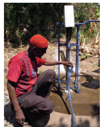
Attache a funnel and a hose to outlet of RP
