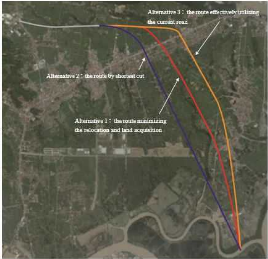
Figure 1.2. Alignment alternatives of Ring Road No. 3
