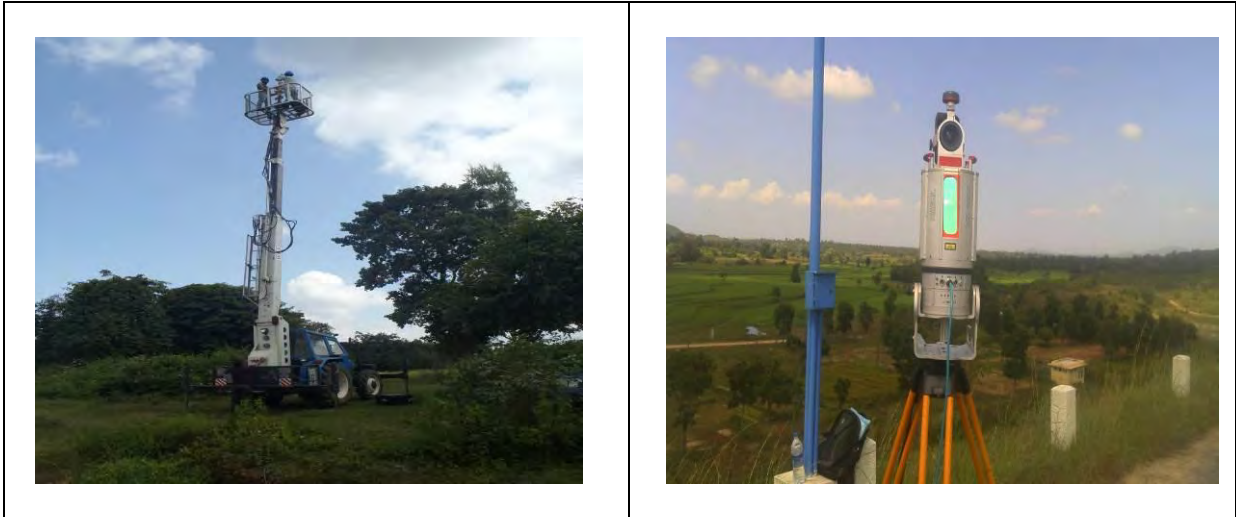
Images Showing Erecting of Terrestrial Lidar system on Tractor elevated Platform
