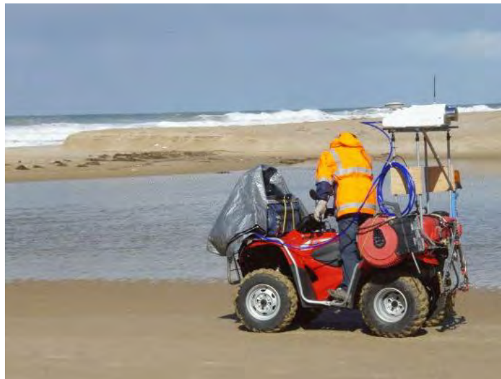
Figure 6-13: Mobile LiDAR Survey using ATV.
