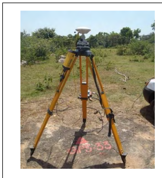
Images Showing Base station setup on the Control point GPS33 site condition at ch19500m
