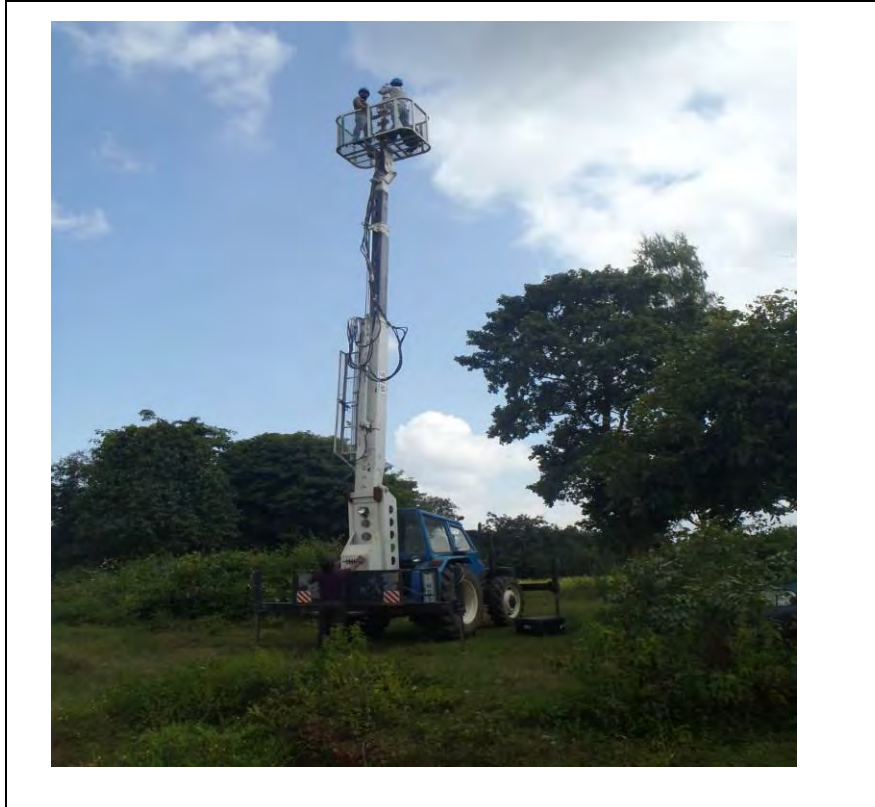
Images Showing Terrestrial Scanner Erected at Site- At Ch 101+000 Km
