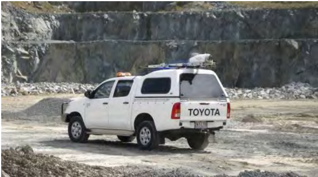
Figure 6-10: Mobile LiDAR Survey
