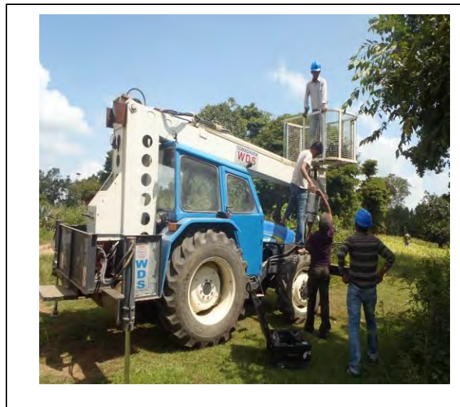
Images Showing Erecting of Terrestrial Lidar system on Tractor elevated Platform
