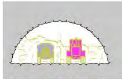
Fig.2 Mucking using loader and dumper
