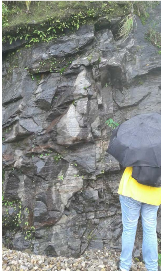
Figure 10 : Granite Gneiss, Unweathered to slightly weathered
