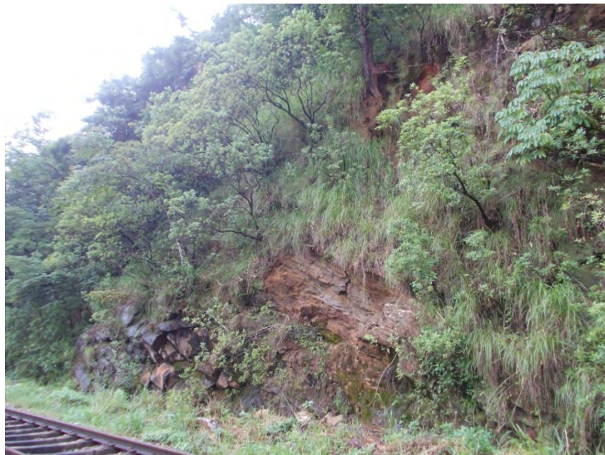
Figure 11 : Granite Gneiss, moderately to highly weathered
