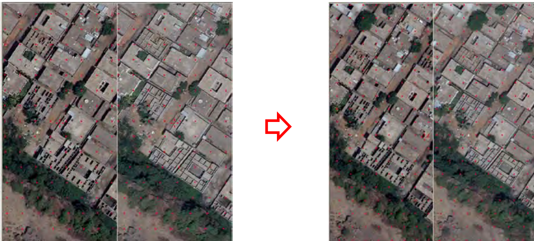
Figure 4-14 Stereo Images in DEM Editing (Before Editing (Left) and After Editing (Right))
