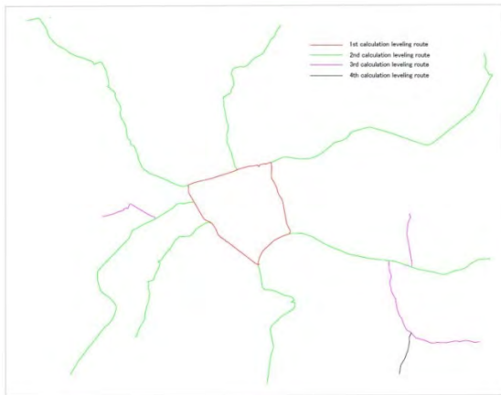
Figure 3-8 Calculation Order for Elevations of Leveling Routes
