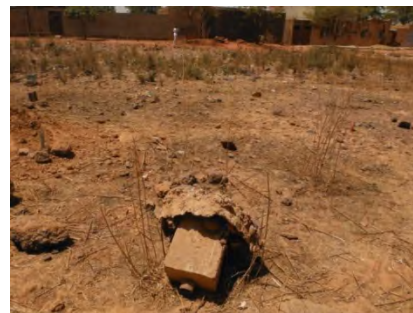
Broken condition of geodetic point (T58)
