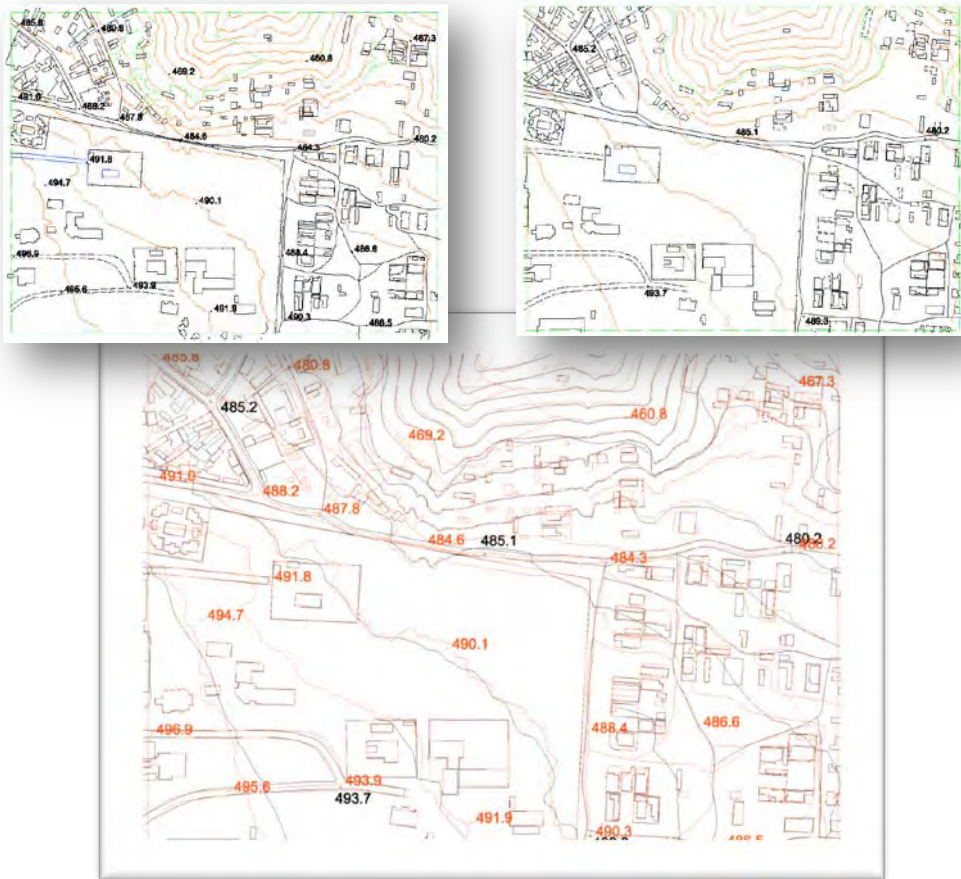
Figure 4-3 Map Created by Overlapping the Plotting Data from Practical Training with Standard Plotting Data (Bottom)
