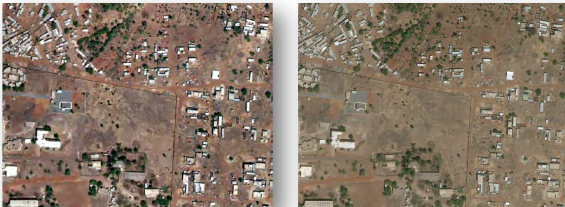
Figure 4-2 (a) Orthophoto Image produced by trainees, (b) Orthophoto Image produced in Japan
