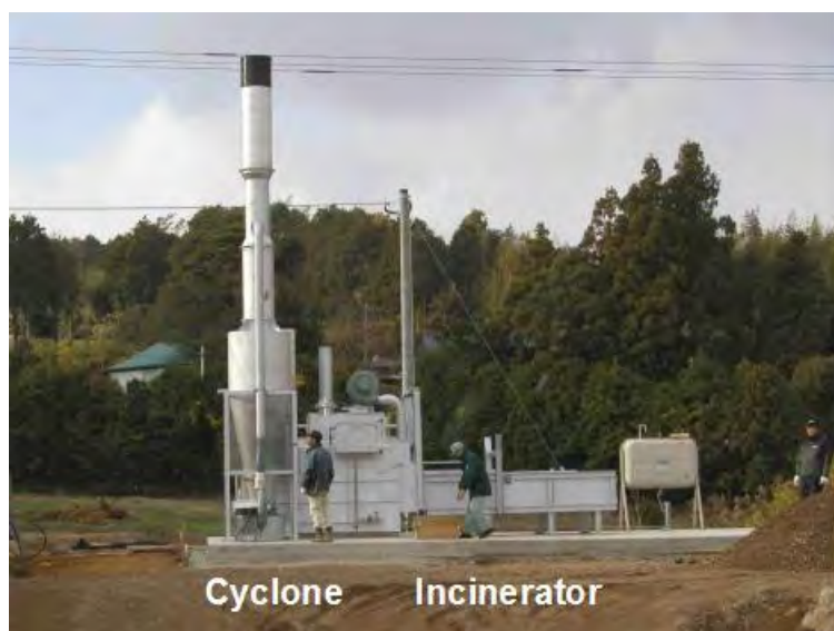
Picture 1 Waste Incinerator MA-Y200 (Installation Example in Japan)
