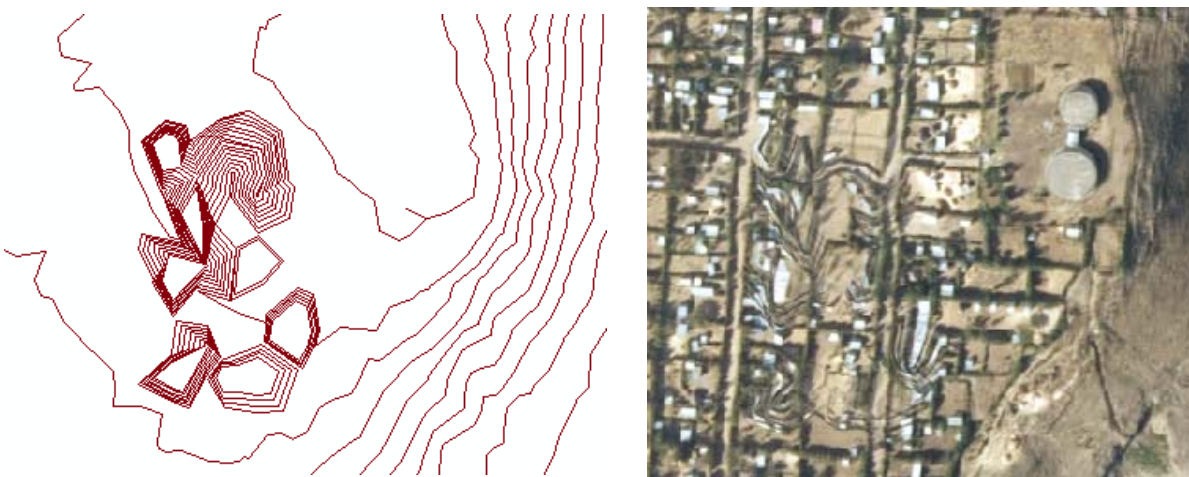
Figure 28 Examples of Errors in Ortho Images (Left: DTM; Right: Orthophoto)
