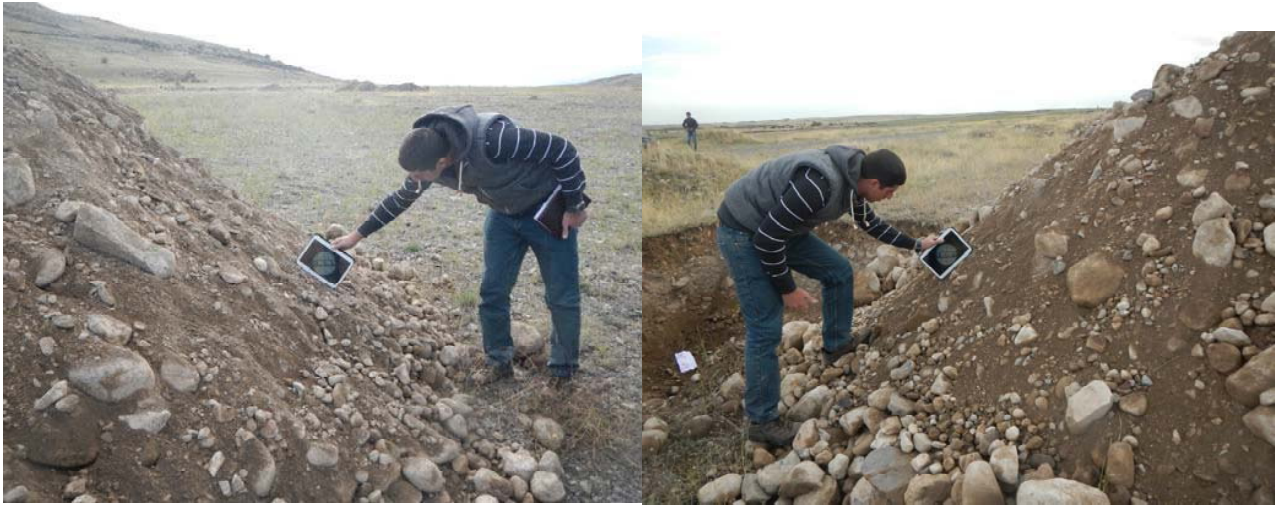
Figure 8. Measurement of the repose angle
