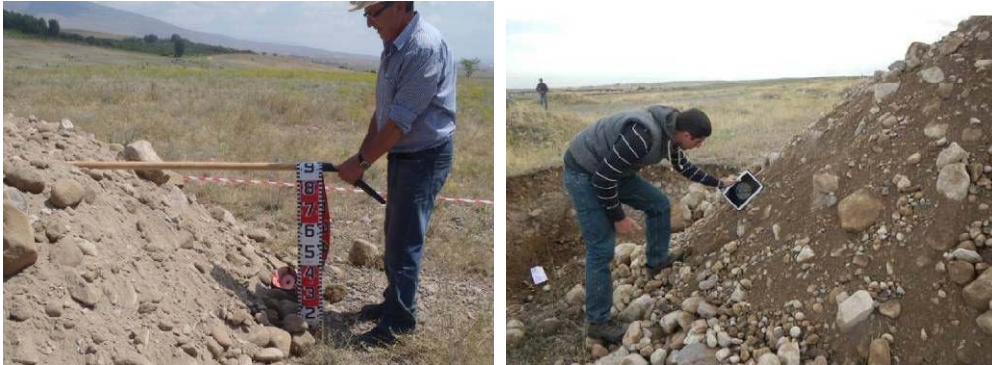
Figure 4-3-7.7 Circumstances in the Repose Angle Measurement
