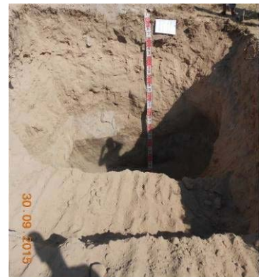
Figure 4-3-4.9 Test-pit Excavated into Volcanic Sand
