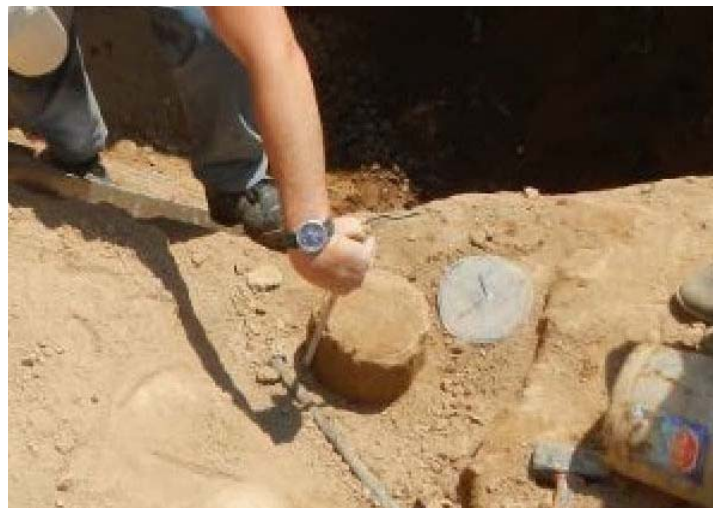
Figure 17. Scraping out and shaping of the soil column
