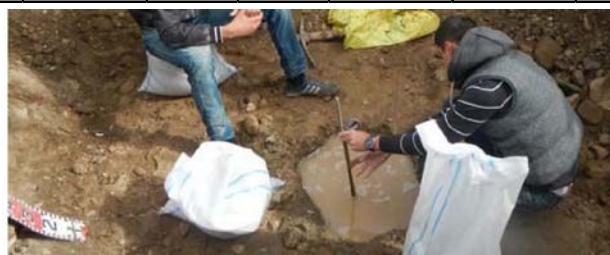
Figure 4-3-7.6 Circumstances in the Field Permeability Test
