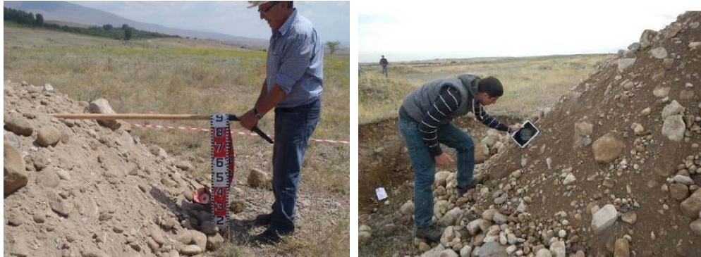
Figure 4-3-7.7 Circumstances in the Repose Angle Measurement
