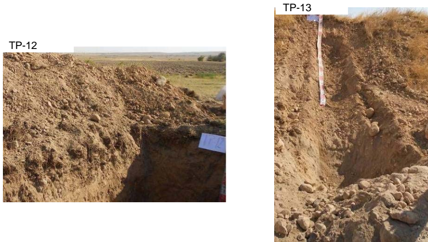
Figure 4-3-4.12 Sand-and-gravel with Rich Silty Sand
