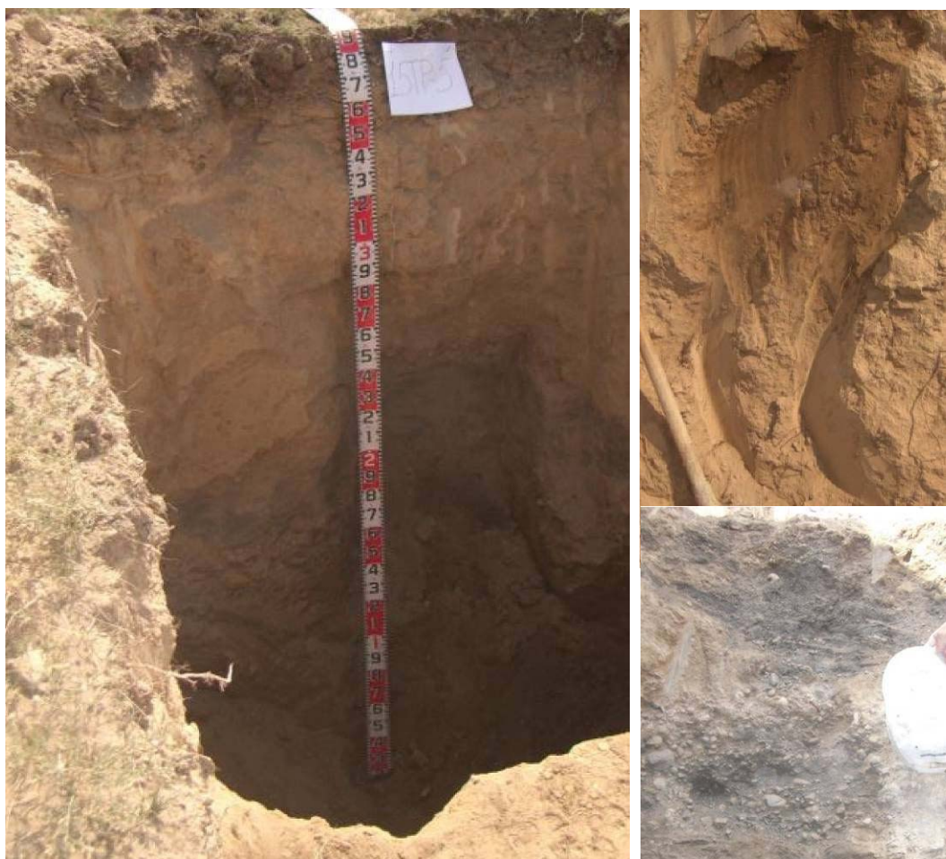
Figure 4-3-4.2 Typical Test Pit Log and the Profile Photos
