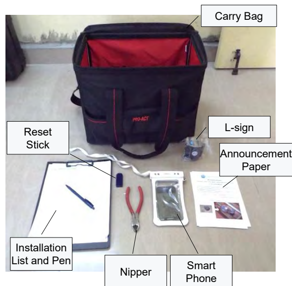
Figure 3-12 Preparation for L-sign installation
