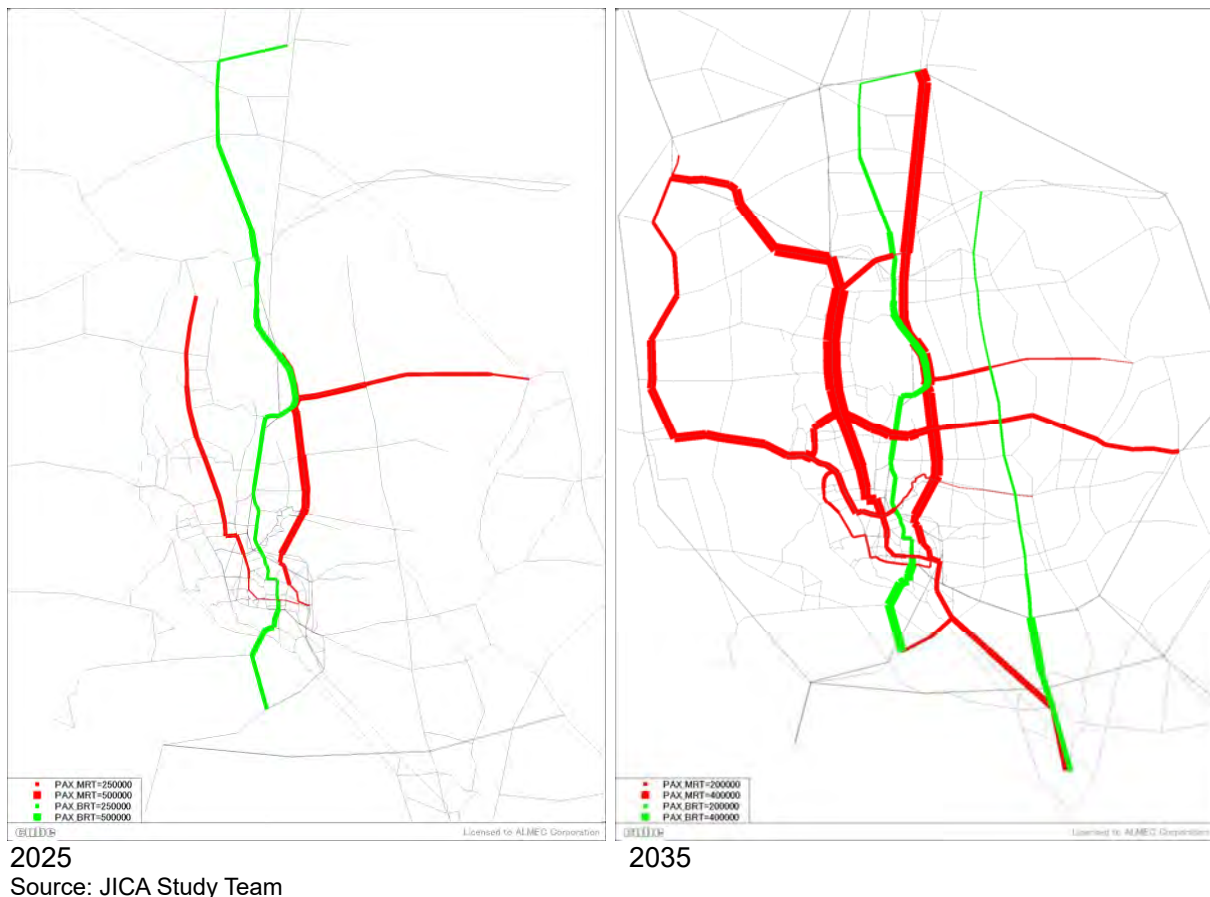
Figure 13.2 Estimated MRT/BRT Traffic in 2025 and 2035
