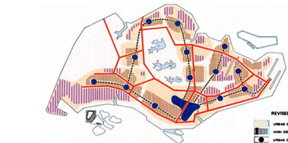
Singapore Conceptual Plan (High-density new town development integrated with UMRT and Urban Expressway)
