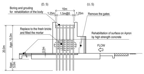
Fig 4.2.8 Example for the rehabilitation of the existing DGR
