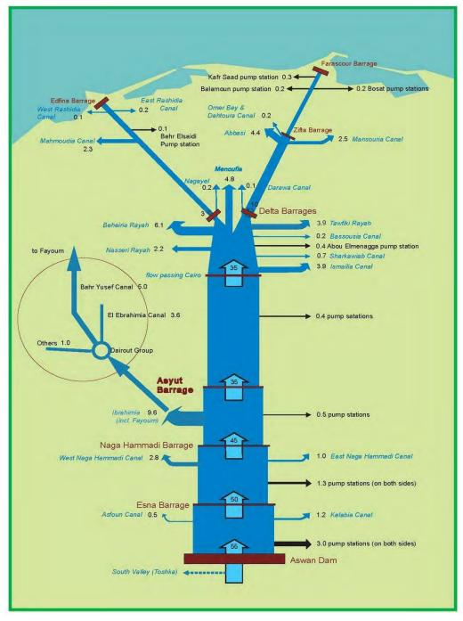
Figure 2.2.1 Water distribution Nile System (source; NAWQAM project)
