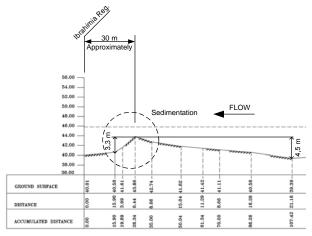
Figure 3.3.15 Longitudinal Profile of Upstream Ibrahima Canal
