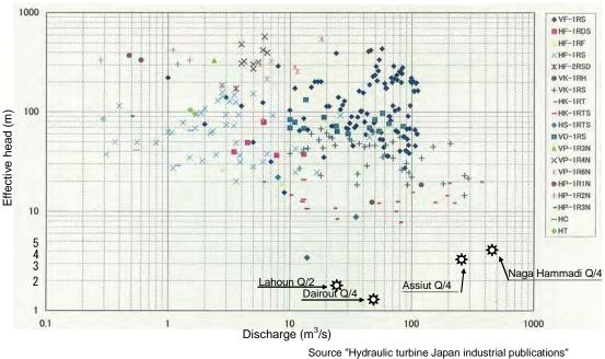
Fig 4.2.9 Empirical results of turbine types in Japan
