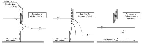
Figure 3.3.6 operation of the three leaf gate
