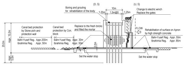
Figure 3.3.24 Rehabilitation of the DGR on standard section
