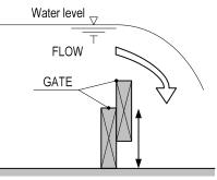
Figure 4.2.5 Discharge by Over-flow Type Gate
