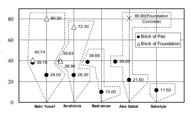
Figure 3.3.18 Distribution of the compressive strength of the inside regulator
