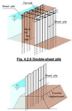
Fig. 4.2.7 Single-sheet pile
