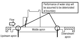
Figure 3.3.20 Assumed position of the damaged water stop
