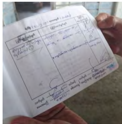
Contents of the journal on the left (From left to right, person reporting the fault, description of the fault, person who took remedial action)
