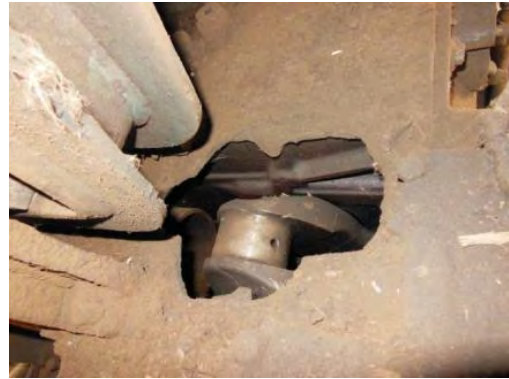
Piston connecting rod breaking through the cover after coming off
