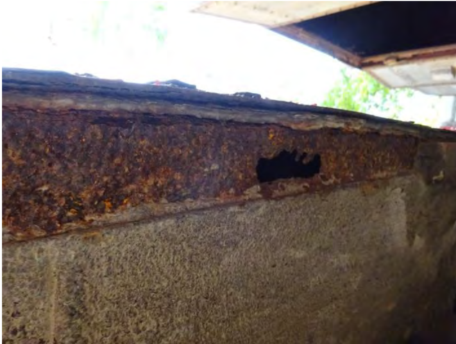
Figure 4-3-1 Underframe in rusted and perforated state
