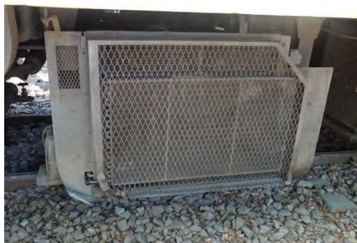
Equipment deformed as a result of collision
