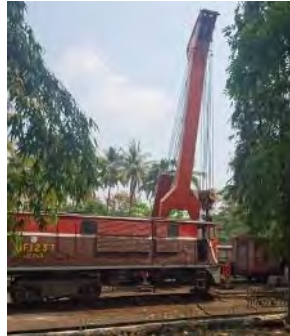
Crane (substitute for lifting jack)
