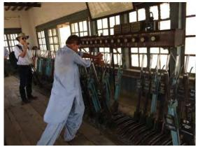
Source: JICA Study Team Figure 2-20 Operation of Mechanical Interlocking
