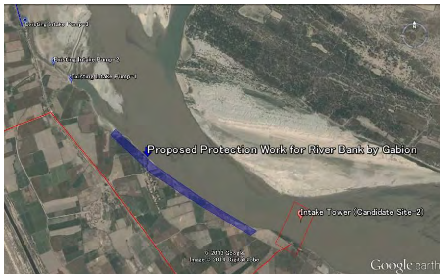
Figure 7.3-38 Locations of Proposed Site of the River Bank Protection
