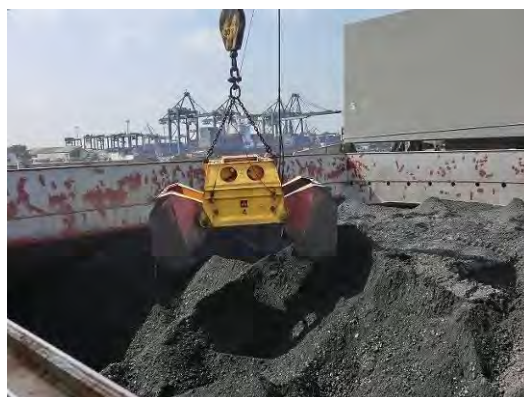
Photo 5.3-2 Grab Unloader (4 ton) Equipped on Vessel
