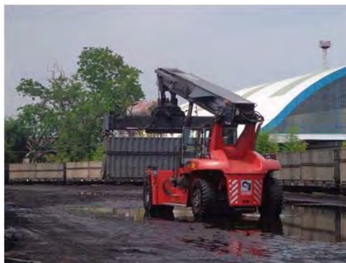
Figure 5-4 Unloading of Coal Container by Reach Stacker (Indonesia)
