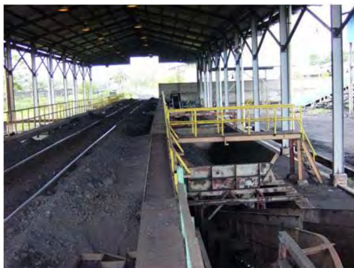
Figure 6-15 Coal Pit for Side/Bottom Hopper Wagon
