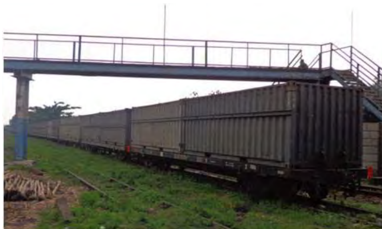
Figure 5-2 An Example of 20 ft Containers Transported by a Coal Wagon
