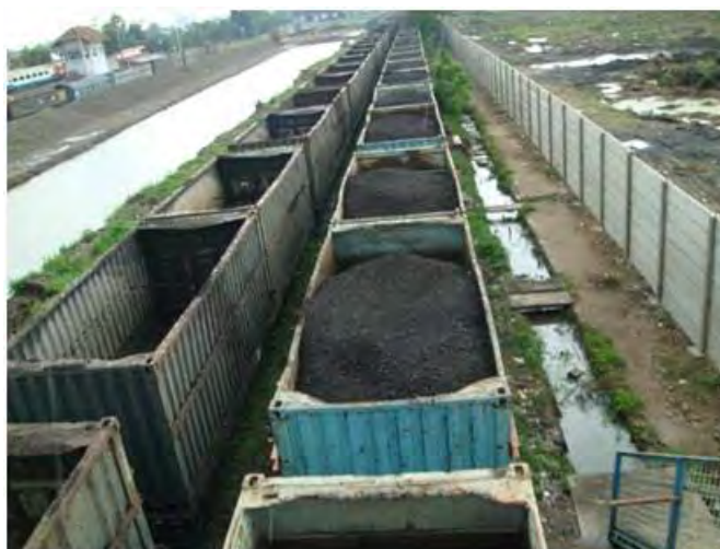
Figure 5-3 Open-Top Coal Container (Indonesia)
