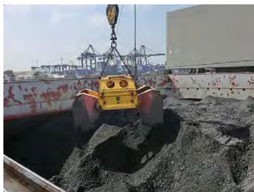
Photo 5.3-2 Grab Unloader (4 ton) Equipped on Vessel
