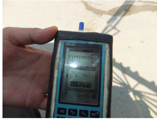
Hand-held Device for Water Meter Reading
