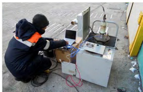
8 Filter regeneration test out doors in winter
