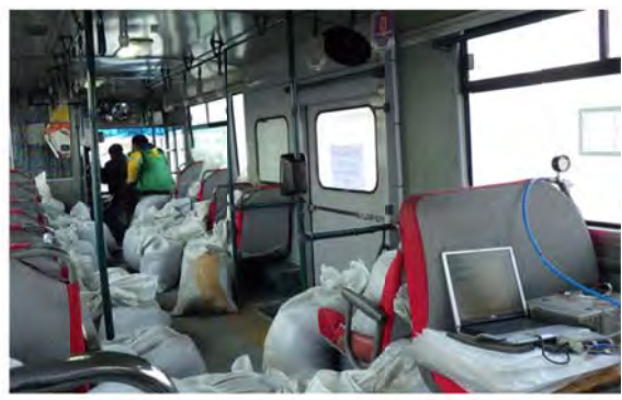
4 Inside of Daewoo bus for running test
