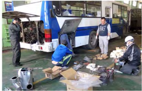
2 Installation of DPF (MoCobee) to Daewoo Bus
