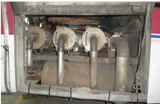
3 DPF (MoCobee) installed to Daewoo bus
