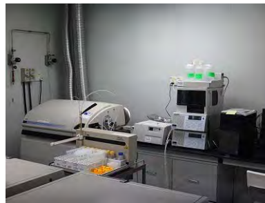
LC-ICP-MS for MeHg (Public Health Lab, MOH)
