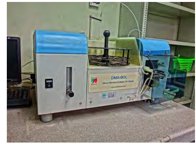
Hg analyzer (Milestone DMA-80L)
