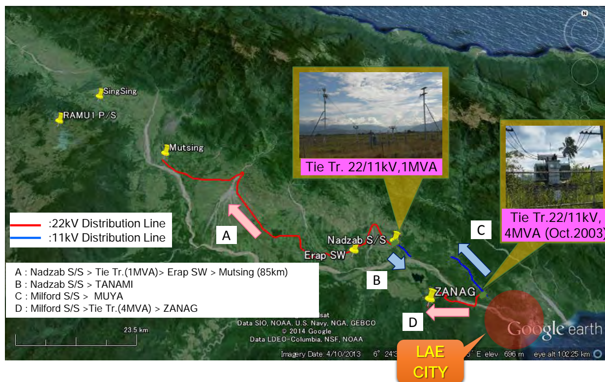
Fig. 2.1-6 Distribution Line in the Lae Area
