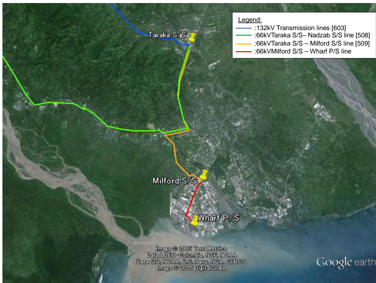
Fig. 2.1-2 66kV Transmission Lines Route
