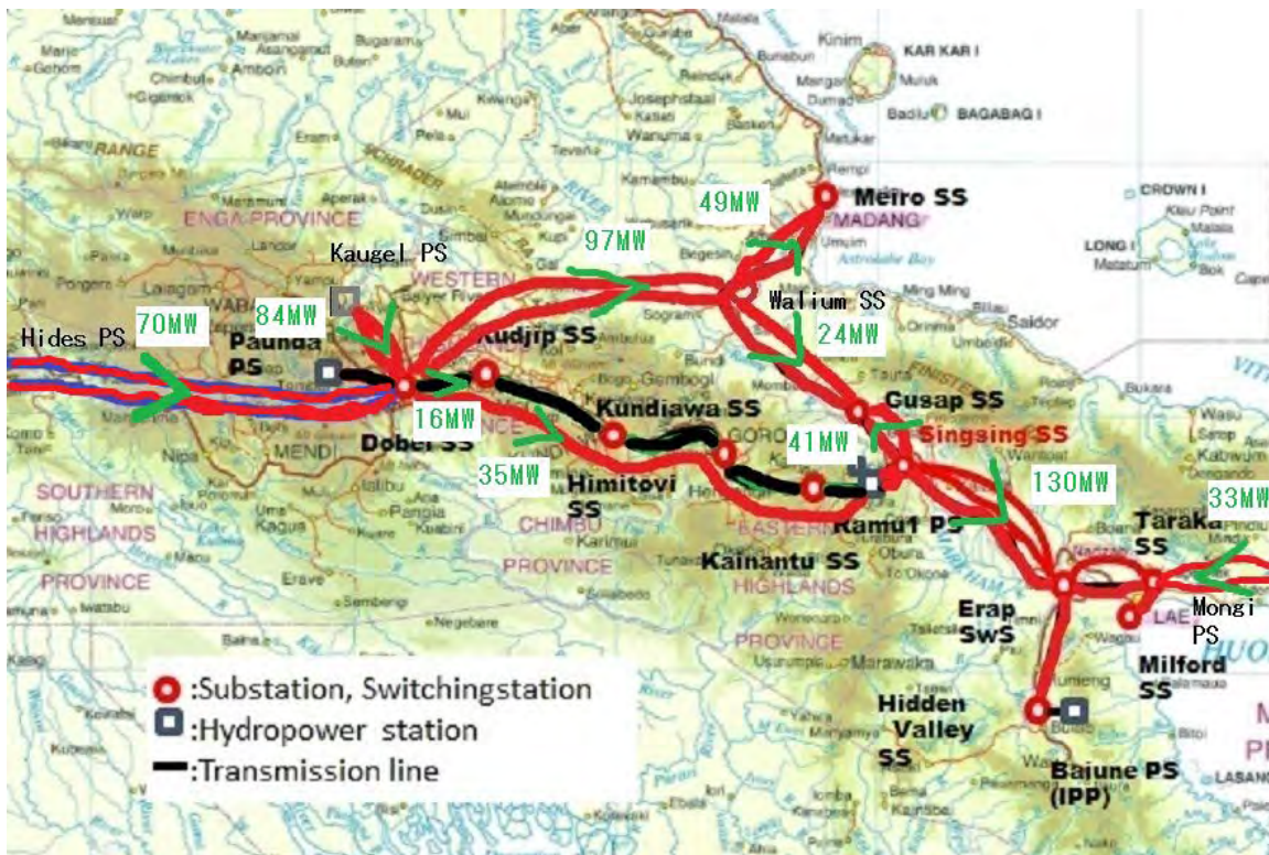
Fig. 7.7-38 Outline of the Power Flow State at the Time of 70 MW Transmission
