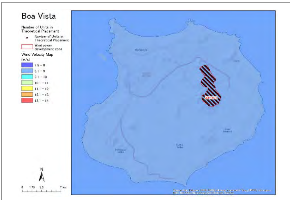
Figure 7.3-31 Theoretical arrangement of windmills in the wind-power generation development zone in Boa Vista (development zone: 1 location)
