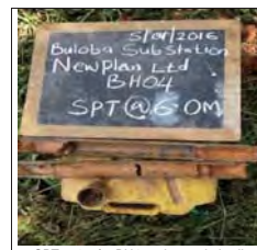
SPT at 6m for BH4, moist mottled yellowish brown firm intact clay of low plasticity, lean clay
