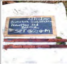
SPT@2m for BH2, moist reddish brown stiff intact silt of high plasticity, elastic silt
