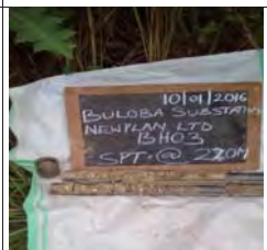
SPT at 22m for BH3, moist yellowish grey stiff intact silt of high plasticity, elastic silt
