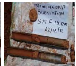
Very Stiff, Moderate Orange Pink, moist, Sandy Elastic SILT soil drilled from BH1 at a depth of 15.0-15.5 m
