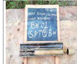
SPT at 3m for BH1, moist brownish grey medium dense granular clayey sand
