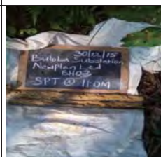
SPT at 11m for BH3, moist mottled brownish yellow firm intact silt of high plasticity, elastic silt
