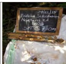
SPT at 7m for BH3, moist greyish yellow firm intact silt of high plasticity, elastic sandy silt
