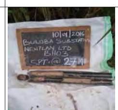
SPT at 27m for BH3, very dense reddish yellowish grey silt of high plasticity, elastic silt
