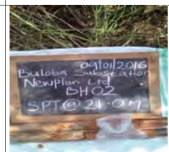
SPT at 21m for BH2, Moist mottled yellowish brown stiff intact silt of high plasticity, elastic silt
