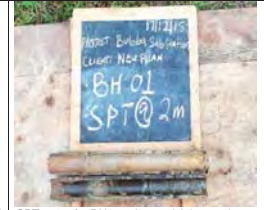
SPT at 2m for BH1, moist greyish brown loose granular clayey sand soil
