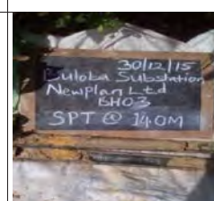
SPT at 14m for BH3, moist mottled brownish yellow firm intact silt of high plasticity, elastic silt
