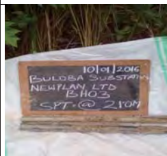
SPT at 21m for BH3, moist yellowish grey stiff intact silt of high plasticity, elastic silt
