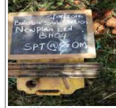
SPT at 8m for BH4, moist greyish brown clay of low plasticity, lean clay
