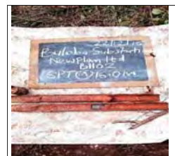
SPT at 16m for BH2, moist mottled reddish stiff intact silt of high plasticity, elastic silt
