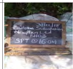
SPT at 16m for BH3, moist mottled brownish yellow firm intact silt of high plasticity, elastic silt
