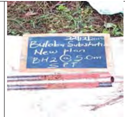
SPT at 5m, moist reddish brown stiff intact silt of high plasticity, elastic silt
