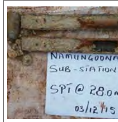
Highly weathered, Pink, Greenish Grey, Coarse grained Weak Rock drilled from BH1 at a depth of 28-28.5 m
