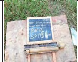
SPT at 4m for BH1, moist greyish yellow firm intact silt of high plasticity, elastic silt
