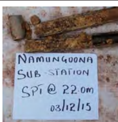
Hard, Mottled Yellowish Grey, moist Sandy SILT soils drilled from BH1 at a depth of 22-22.5 m
