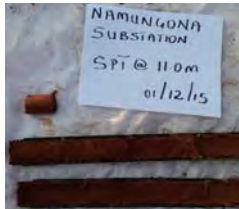
Stiff, Moderate Reddish Brown, moist, Sandy Fat CLAY drilled from BH1 at a depth of 11-11.5 m
