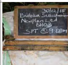
SPT at 9m for BH3, moist yellowish brown dense granular clayey sand
