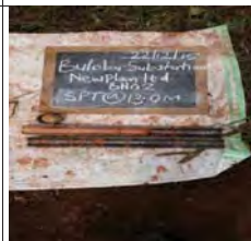
SPT at 13m for BH2, moist mottled yellowish brown stiff intact silt of high plasticity, elastic silt
