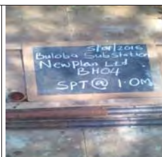
SPT at 1m for BH4, Moist reddish brown soft intact clay of high plasticity, flat clay
