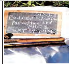
SPT at 1m for BH3, moist greyish brown very loose granular clayey sand
