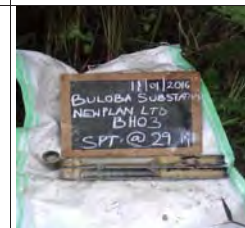
SPT at 29m for BH3, very dense reddish yellowish grey silt of high plasticity, elastic silt
