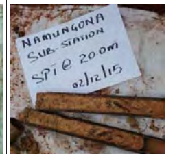
Hard, Moderate Yellow, moist, Sandy Elastic SILT soils drilled from BH1 at a depth of 20-20.5 m
