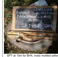
SPT at 10m for BH4, moist mottled yellowish brown firm intact silt of high plasticity, elastic silt
