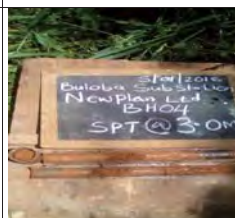
SPT at 3m for BH4, moist reddish brown soft intact silt with
