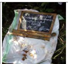
SPT at 6m for BH3, moist greyish yellow firm intact silt of high plasticity, elastic sandy silt
