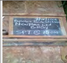
SPT at 15m for BH4, moist mottled greyish yellow stiff intact silt of high plasticity, elastic silt
