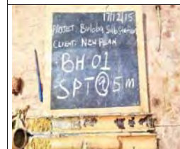
SPT at 5m for BH1, moist greyish yellow firm intact clay of low plasticity, lean clay
