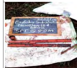
SPT at 6m for BH2, moist mottled reddish brown medium dense silty gravel with sand
