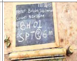
SPT at 6m for BH1, moist greyish yellow medium dense granular elastic sandy silt
