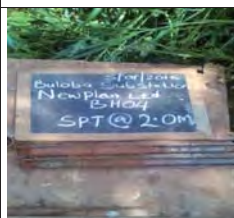
SPT at 2m for BH4, moist reddish brown soft intact clay of high plasticity, flat clay
