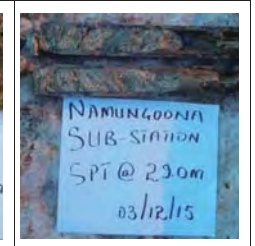
Highly weathered, layered, Pink, Greenish Grey, Weak ROCK and Clayey SAND infill soil drilled from BH1 at a depth of 29.0-29.5 m
