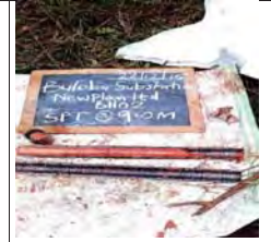
SPT at 9m for BH2, moist mottled reddish firm intact silt of high plasticity, elastic sandy silt
