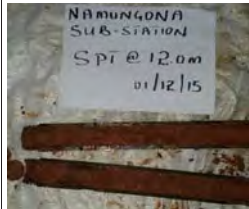
Medium Dense, Moderate Reddish Brown, coarse grained clayey SAND soils drilled from BH1 at a depth of 12-12.5 m
