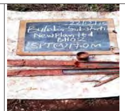
SPT at 17m for BH2, moist mottled reddish stiff intact silt of high plasticity, elastic silt
