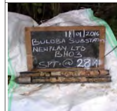
SPT at 28m for BH3, very dense reddish yellowish grey silt of high plasticity, elastic silt
