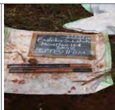
SPT at 11m for BH2, moist mottled reddish brown firm intact clay of low plasticity, lean clay
