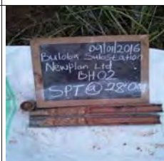
SPT at 28m for BH2, moist mottled yellowish brown stiff intact silt of high plasticity, elastic silt
