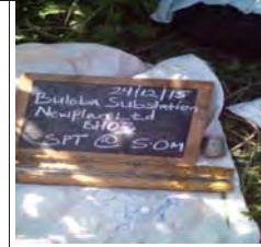
SPT at 5m for BH3, moist greyish yellow firm intact silt of high plasticity, elastic sandy silt
