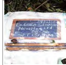
SPT at 4m for BH3, moist mottled yellowish brown firm intact clay of high plasticity, flat clay
