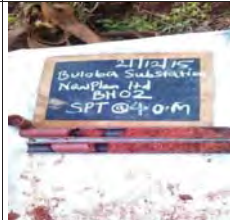
SPT at 4m for BH2, moist reddish brown stiff intact silt of high plasticity, elastic silt
