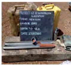
Moist reddish brown stiff homogeneous silty sandy CLAY drilled from BH1 at a depth of 9.0-9.5 m
