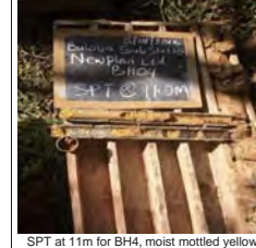
SPT at 11m for BH4, moist mottled yellowish brown firm intact silt of high plasticity, elastic silt
