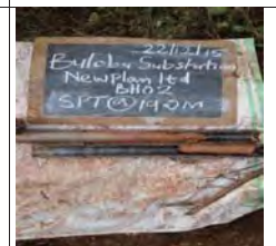
SPT at 19m for BH2, moist mottled yellowish brown stiff intact silt of high plasticity, elastic silt
