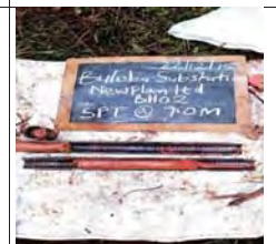
SPT@7m for BH2, moist mottled yellowish brown firm intact silt of high plasticity, elastic sandy silt
