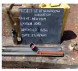
Moist reddish brown stiff homogeneous silty sandy CLAY drilled from BH1 at a depth of 10.0-10.5 m
