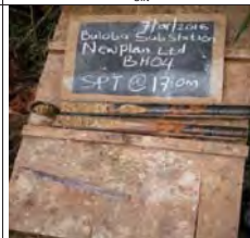
SPT at 17m for BH4, moist mottled greyish yellow stiff intact silt of high plasticity, elastic silt
