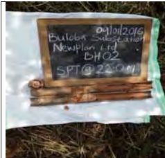
SPT at 22m for BH2, moist mottled yellowish brown stiff intact silt of high plasticity, elastic silt
