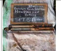
SPT at 19m for BH4, moist mottled greyish yellow stiff intact silt of high plasticity, elastic silt
