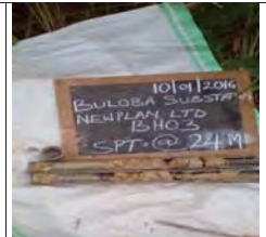
SPT at 24m for BH3, very dense reddish yellowish grey silt of high plasticity, elastic silt
