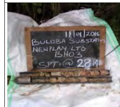
SPT at 28m for BH3, very dense reddish yellowish grey silt of high plasticity, elastic silt
