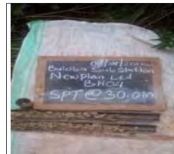
SPT at 30m for BH4, moist mottled greyish brown firm intact silt of high plasticity, elastic silt
