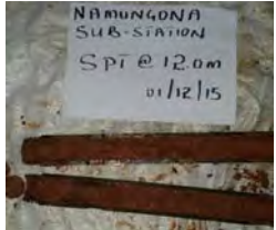
Medium Dense, Moderate Reddish Brown, coarse grained clay SAND soils drilled from BH1 at a depth of 12-12.5 m
