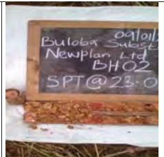
SPT at 23m for BH2, moist mottled yellowish brown stiff intact silt of high plasticity, elastic silt
