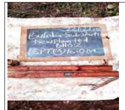
SPT at 16m for BH2, moist mottled reddish stiff intact silt of high plasticity, elastic silt
