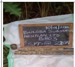
SPT at 22m for BH3, moist yellowish grey stiff intact silt of high plasticity, elastic silt
