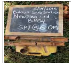
SPT at 6m for BH4, moist mottled yellowish brown firm intact clay of low plasticity, lean clay
