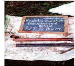
SPT at 8m for BH2, moist reddish firm intact silt of high plasticity, elastic sandy silt
