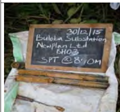
SPT at 8m for BH3, moist brownish yellow stiff intact clay of low plasticity, lean clay
