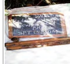
SPT at 3m for BH3, moist greyish brown firm intact clay of low plasticity, lean clay
