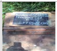
SPT at 5m for BH4, moist reddish brown firm intact clay of high plasticity, flat clay
