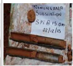
Very Stiff, Moderate Orange Pink, moist, Sandy Elastic SILT soil drilled from BH1 at a depth of 15.0-15.5 m
