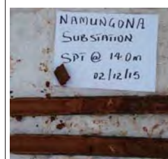
Medium Dense, Moderate Yellow, Coarse grained Clayey SAND with cobbles soils drilled from BH1 at a depth of 14-14.5 m
