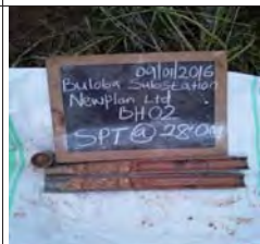
SPT at 28m for BH2, moist mottled yellowish brown stiff intact silt of high plasticity, elastic silt
