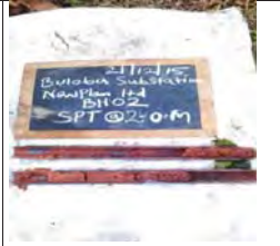
SPT@2m for BH2, moist reddish brown stiff intact silt of high plasticity, elastic silt
