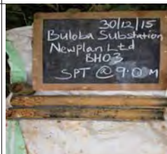
SPT at 9m for BH3, moist yellowish brown dense granular clayey sand
