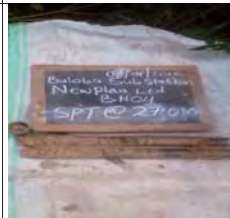
SPT at 27m for BH4, moist mottled greyish brown firm intact silt of high plasticity, elastic silt
