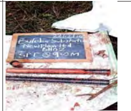
SPT at 9m for BH2, moist mottled reddish firm intact silt of high plasticity, elastic sandy silt
