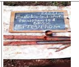
SPT at 17m for BH2, moist mottled reddish stiff intact silt of high plasticity, elastic silt
