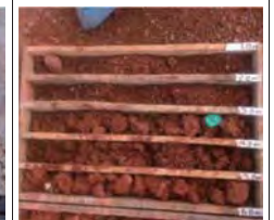
Retrieved Soil samples between 1.0m depth and 6.0m depth. Imported soil layers between 1.0m and 2.5m depth was of Moderate Reddish Brown Clayey SAND soils with Gravel.
