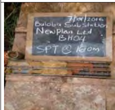
SPT at 16m for BH4, Moist mottled greyish yellow stiff intact silt of high plasticity, elastic silt
