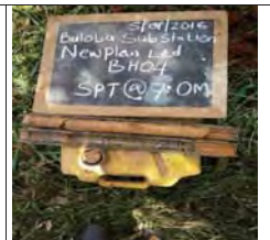
SPT at 7m for BH4, moist mottled yellowish brown firm intact clay of high plasticity, flat clay
