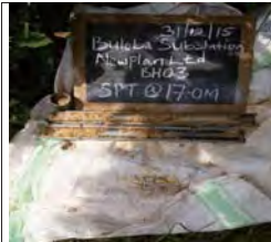
SPT at 17m for BH3, moist mottled brownish yellow firm intact silt of high plasticity, elastic silt
