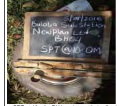
SPT at 10m for BH4, moist mottled yellowish brown firm intact silt of high plasticity, elastic silt
