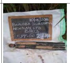
SPT at 27m for BH3, very dense reddish yellowish grey silt of high plasticity, elastic silt
