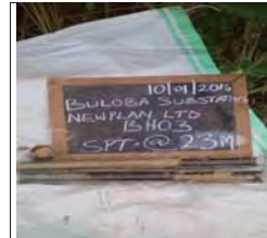
SPT at 23m for BH3, moist yellowish grey stiff intact silt of high plasticity, elastic silt
