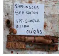
Very Stiff, Mottled Moderate Yellow, sandy Elastic SILT soils drilled from BH1 at a depth of 19-19.5 m
