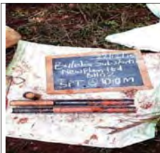
SPT at 10m for BH2, moist reddish brown firm intact silt of high plasticity, elastic silt
