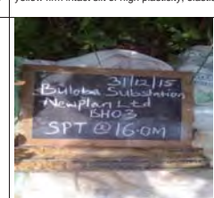
SPT at 16m for BH3, moist mottled brownish yellow firm intact silt of high plasticity, elastic silt
