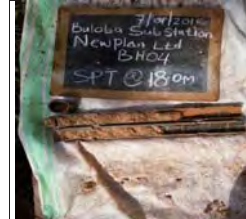
SPT at 18m for BH4, Moist mottled greyish yellow stiff intact silt of high plasticity, elastic silt
