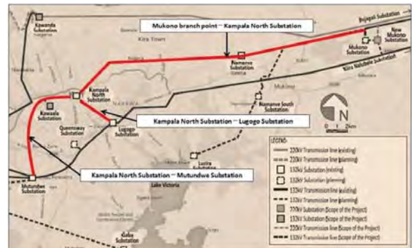
Source: JICA Project Team Figure 2-12: Sections of transmission lines that will be re-conductored (lines in red)
