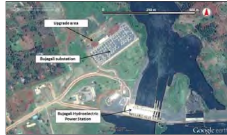
Figure 2-7: Existing topographical layout of Bujagali substation and upgrade area
