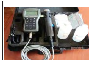
Figure 3-8: Multiparameter water quality meter (HANNA HI 9828) used to measure up to 13 different water parameters
