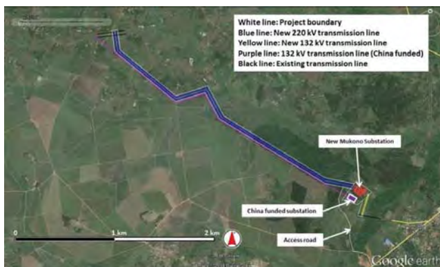
Source: Prepared by JICA Project Team with Google Earth Figure 2-4: Topographical layout of New Mukono substation and associated transmission lines
