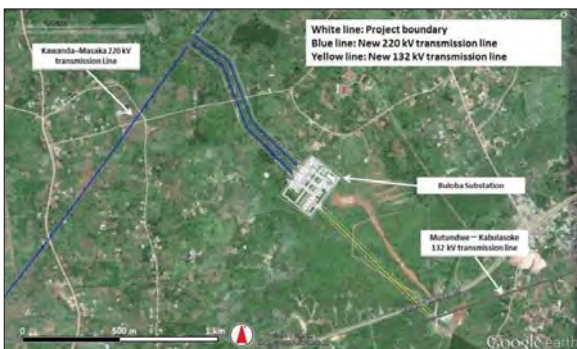
Source: Prepared by JICA Project Team with Google Earth Figure 2-1: Proposed topographical layout of Buloba Substation and associated transmission lines
