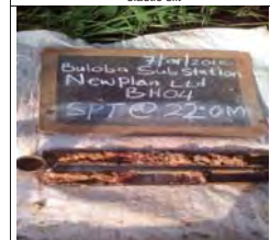
SPT at 22m for BH4, moist mottled greyish brown firm intact silt of high plasticity, elastic silt
