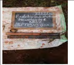
SPT at 13m for BH2, moist mottled yellowish brown stiff intact silt of high plasticity, elastic silt
