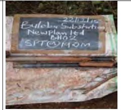
SPT at 19m for BH2, moist mottled yellowish brown stiff intact silt of high plasticity, elastic silt
