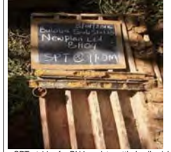
SPT at 11m for BH4, moist mottled yellowish brown firm intact silt of high plasticity, elastic silt
