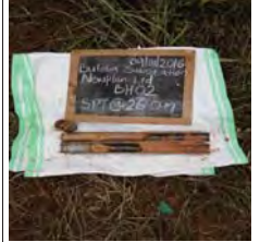
SPT at 26m for BH2, moist mottled yellowish brown stiff intact sandy lean CLAY
