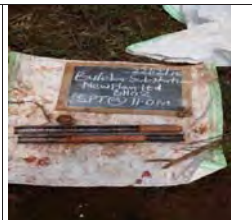
SPT at 11m for BH2, moist mottled reddish brown firm intact clay of low plasticity, lean clay
