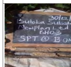
SPT at 13m for BH3, moist mottled brownish yellow firm intact silt of high plasticity, elastic silt
