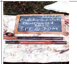
SPT@7m for BH2, moist mottled yellowish brown firm intact silt of high plasticity, elastic sandy silt
