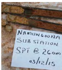
Hard, Yellowish Grey, moist Sandy SILT soil and Residual Rock Material drilled from BH1 at a depth of 26-26.5 m
