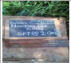
SPT at 2m for BH4, moist reddish brown soft intact clay of high plasticity, flat clay
