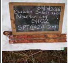
SPT at 24m for BH2, moist mottled yellowish brown stiff intact sandy lean CLAY
