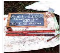
SPT at 6m for BH2, moist mottled reddish brown medium dense silty gravel with sand
