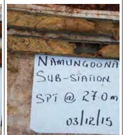
Hard, Yellowish Grey, moist Sandy SILT and Residual Rock material drilled from BH1 at a depth of 27-27.5 m
