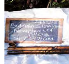
SPT at 2m for BH3, moist greyish brown firm intact clay of low plasticity, lean clay
