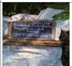
SPT at 11m for BH3, moist mottled brownish yellow firm intact silt of high plasticity, elastic silt
