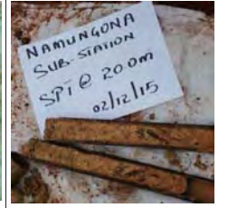
Hard, Moderate Yellow, moist, Sandy Elastic SILT soils drilled from BH1 at a depth of 20-20.5 m
