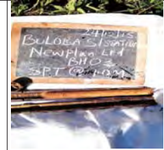
SPT at 1m for BH3, moist greyish brown very loose granular clayey sand
