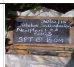
SPT at 14m for BH3, moist mottled brownish yellow firm intact silt of high plasticity, elastic silt
