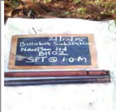
SPT at 1m for BH2, moist reddish brown dense clayey gravel with sand
