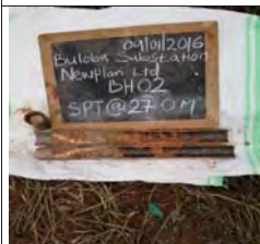
SPT at 27m for BH2, moist mottled yellowish brown stiff intact silt of high plasticity, elastic silt
