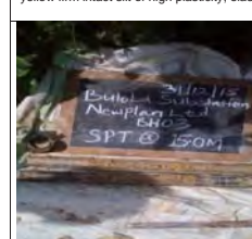
SPT at 15m for BH3, moist mottled brownish yellow firm intact silt of high plasticity, elastic silt
