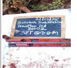
SPT at 4m for BH2, moist reddish brown stiff intact silt of high plasticity, elastic silt
