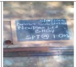
SPT at 1m for BH4, Moist reddish brown soft intact clay of high plasticity, flat clay
