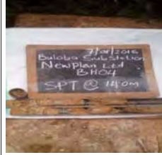
SPT at 14m for BH4, moist mottled greyish yellow stiff intact silt of high plasticity, elastic silt
