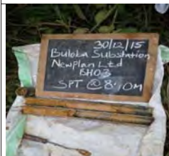
SPT at 8m for BH3, moist brownish yellow stiff intact clay of low plasticity, lean clay
