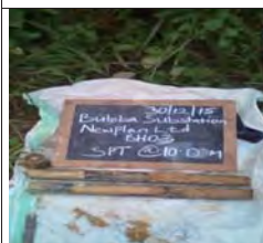
SPT at 10m for BH3, moist yellowish brown medium dense clayey sand
