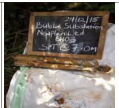
SPT at 7m for BH3, moist greyish yellow firm intact silt of high plasticity, elastic sandy silt
