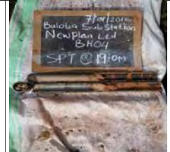
SPT at 19m for BH4, moist mottled greyish yellow stiff intact silt of high plasticity, elastic silt
