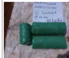
Packed and sealed Un disturbed soil samples retrieved at 15.0m depth for the Triaxial and consolidation tests from BH1 at a depth of 15-15.5 m
