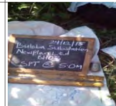
SPT at 5m for BH3, moist greyish yellow firm intact silt of high plasticity, elastic sandy silt
