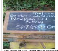
SPT at 9m for BH4, moist greyish yellow stiff intact silt of high plasticity, elastic silt
