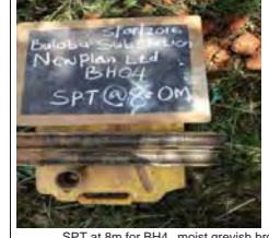
SPT at 8m for BH4, moist greyish brown clay of low plasticity, lean clay
