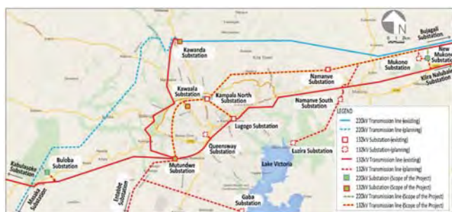
Source: JICA Study Team Figure 1: Transmission Line Network in GKMA (Existing and Planned)
