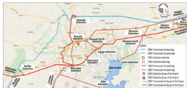
Source: JICA Study Team Figure 1-1: Transmission Line Network in GKMA (Existing and Planned)
