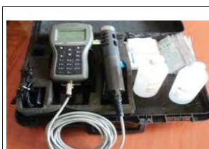
Figure 3-8: Multiparameter water quality meter (HANNA HI 9828) used to measure up to 13 different water parameters
