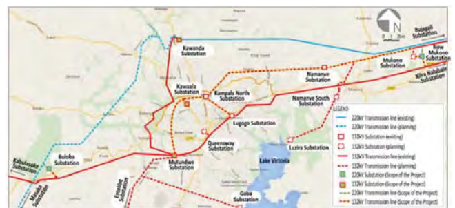
Source: JICA Study Team Figure ES 01: Transmission Line Network in GKMA (Existing and Planned)
