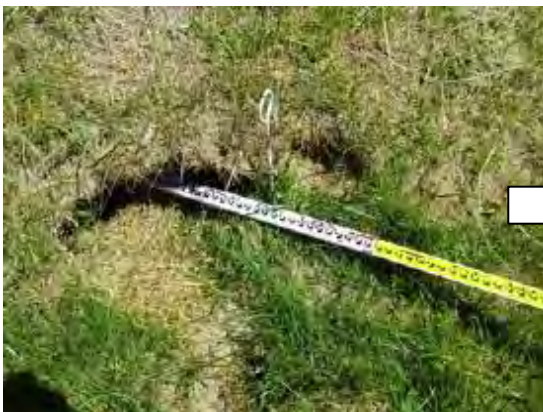
a) Depth of Cavity more than 4 cm
