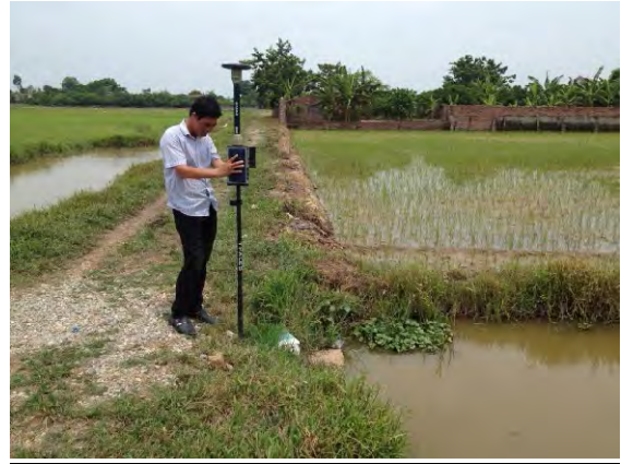
Figure 10 Example of taking elevation by equipment Zmax serving for identifying flood mark
