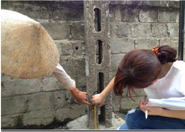
Figure 9 Example of measuring inundation level
