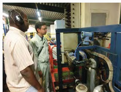
Fuel consumption measurement test (Fuel flow meter measurement)
