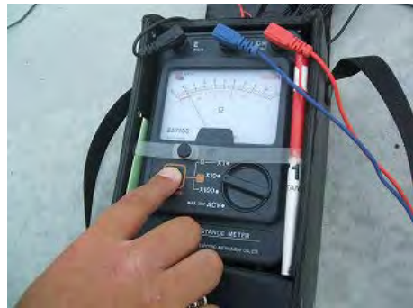
Measurement of grounding resistance
