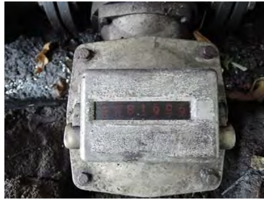
Figure 3.2.5-13 Fuel flow meter (SET M6)
