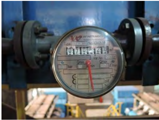
Figure 3.2.5-12 Fuel flow meter (SET 6P-8P)
