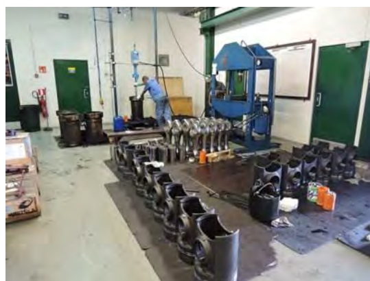
Figure 3.2.5-3 Piston liner processing
