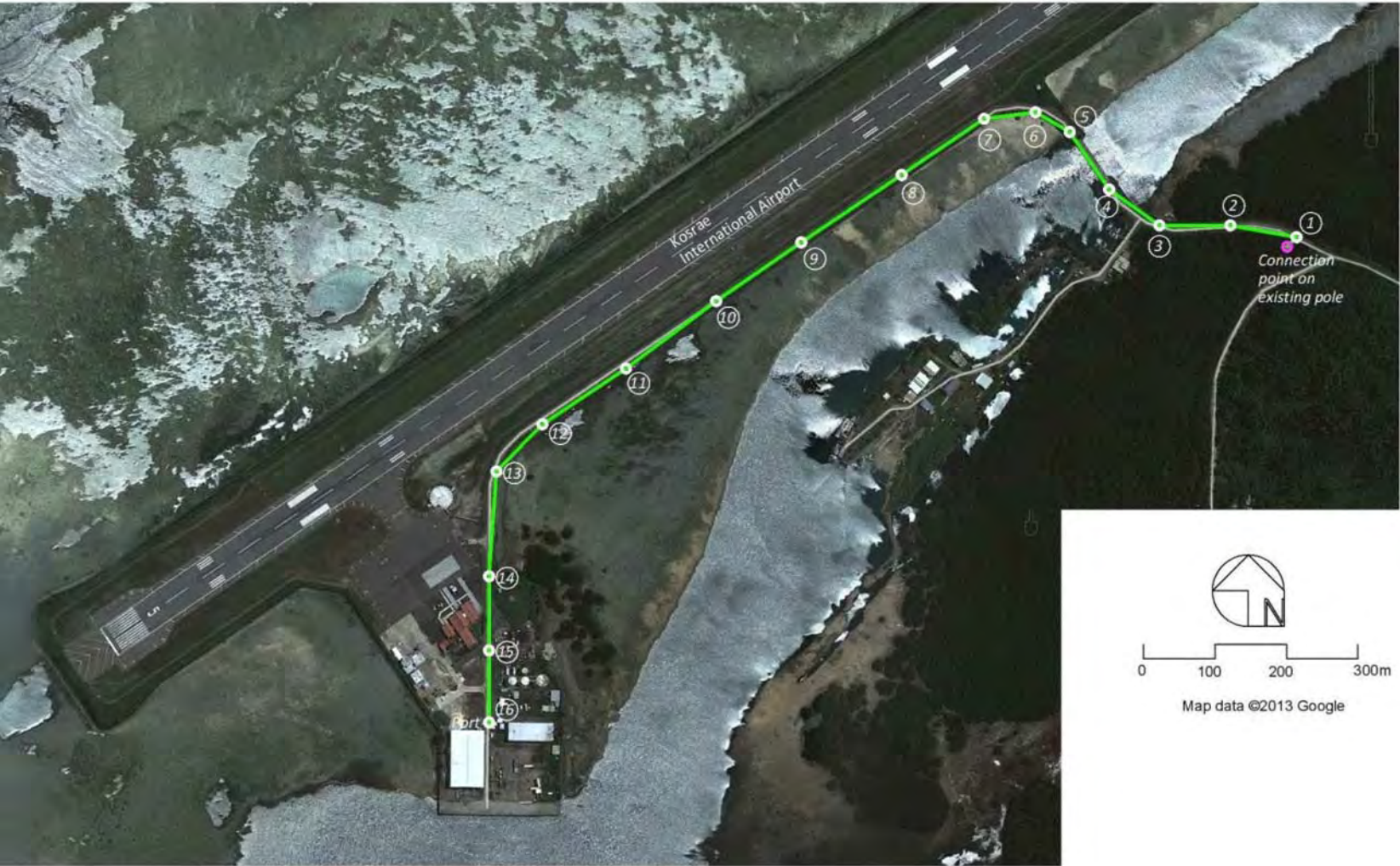
DWG No. UG-R-01 Underground Cable Route Diagram
