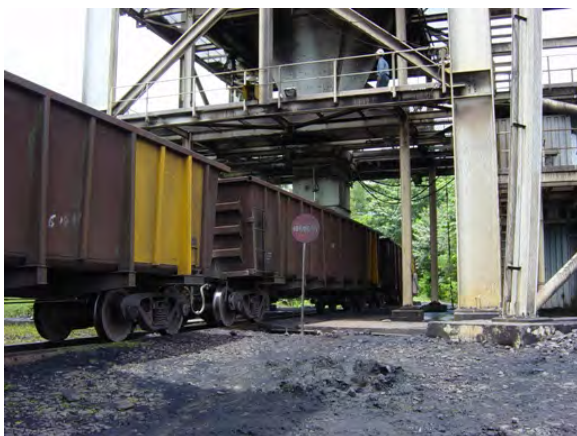
Figure 3.2: Loading of Hopper Wagons by Coal Loading Facility
