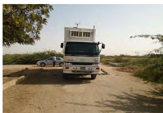
Ambient air quality measurement truck at A02. Area for the proposed coal loading terminal next to PSM can be seen in the background.
