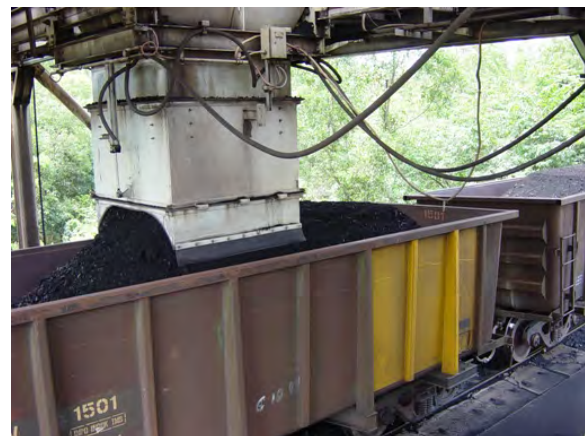
Figure 3.2: Loading of Hopper Wagons by Coal Loading Facility
