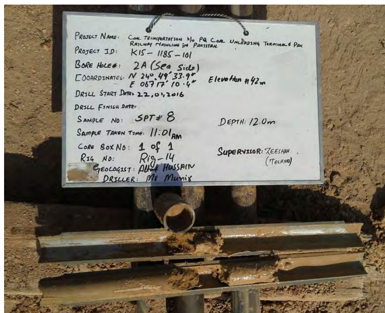
Figure A-3 Disturbed Soil Sample in Split Spoon Sampler
