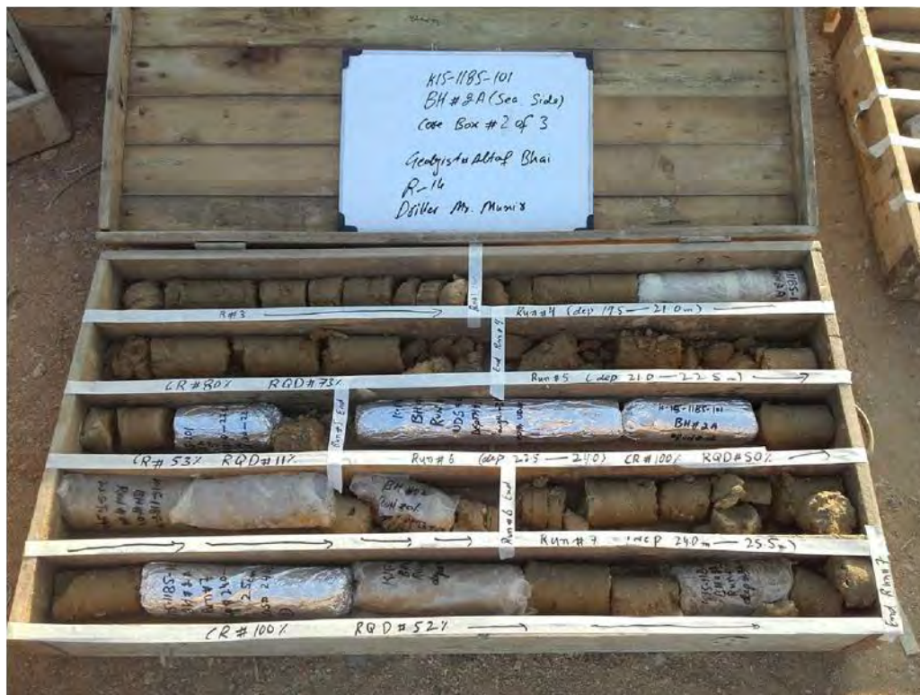
Figure A-4 Rock core samples in core box
