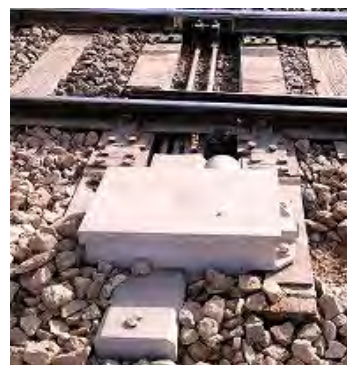
Figure 6-6 Relay Type Interlocking and Electric Point Machine
