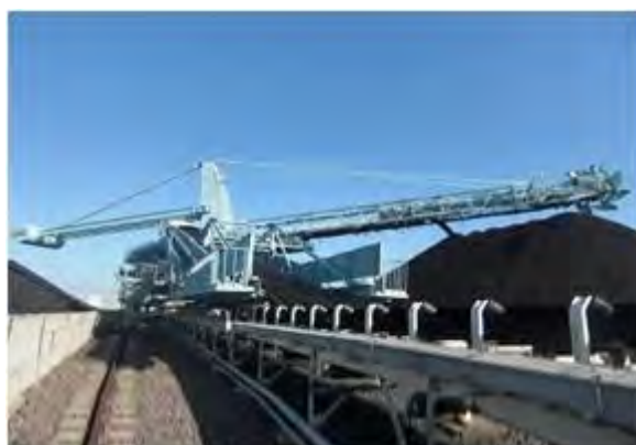
Figure 4-18 Stacker Reclaimer and Dust Suppression Net
