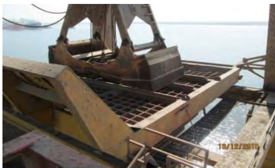
Figure 4-6 27.5 ton Grab Bucket and Receiving Hopper and Conveyor Belt at PSM Land
