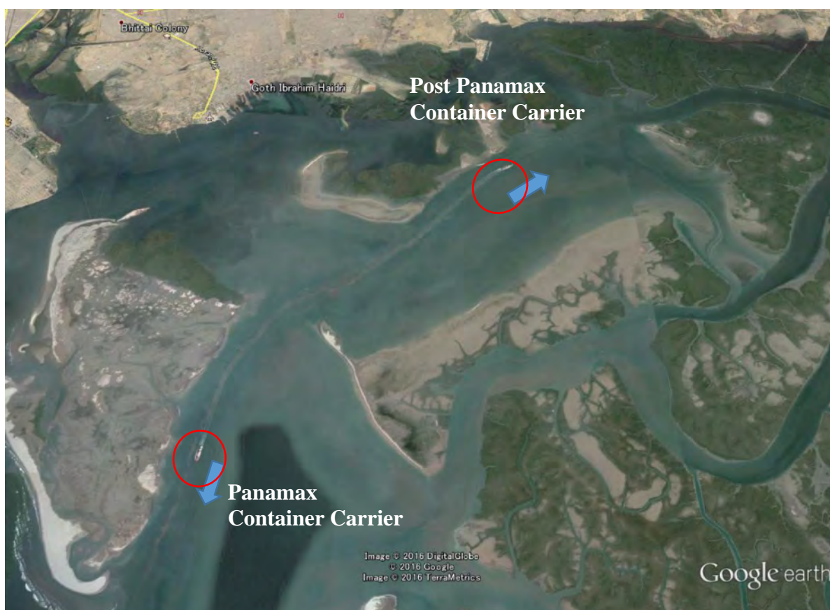
Figure 3-8 Two Ships Moving along One-way Navigation Channel at the Same Time Toward Opposite Directions
