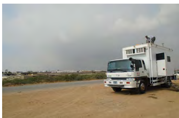
Ambient air quality measurement truck at A01. Bhains Colony can be seen in the background.
