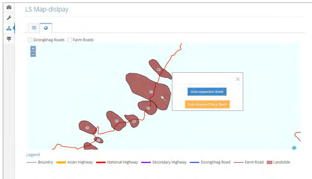
Figure 5.2.13 Sample of Landslide GIS Map Linked with Inspection and Regular Check Sheet (Source: JET)
