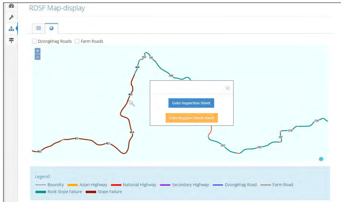
Figure 5.2.15 Sample of Debris Slope Failure and Rock Slope Failure GIS Map Linked with Inspection and Regular Check Sheet (Source: JET)
