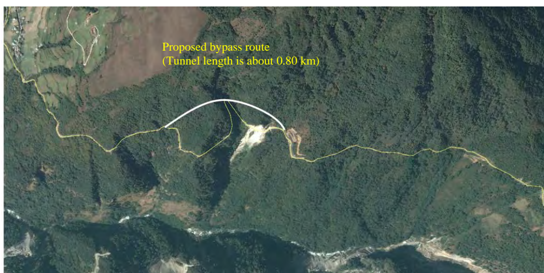
Figure 6.2.5 Proposed Bypass Route at Thumang Cliff (Source: JET)
