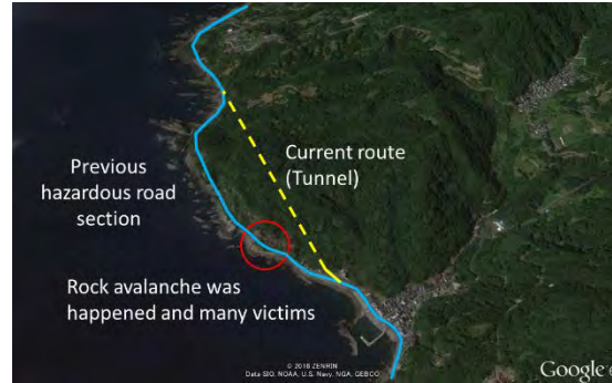
Figure 2.4.10 Case Example of Road Alignment Change due to Slope Disaster in Japan (Source: JET, base map is Google Earth)
