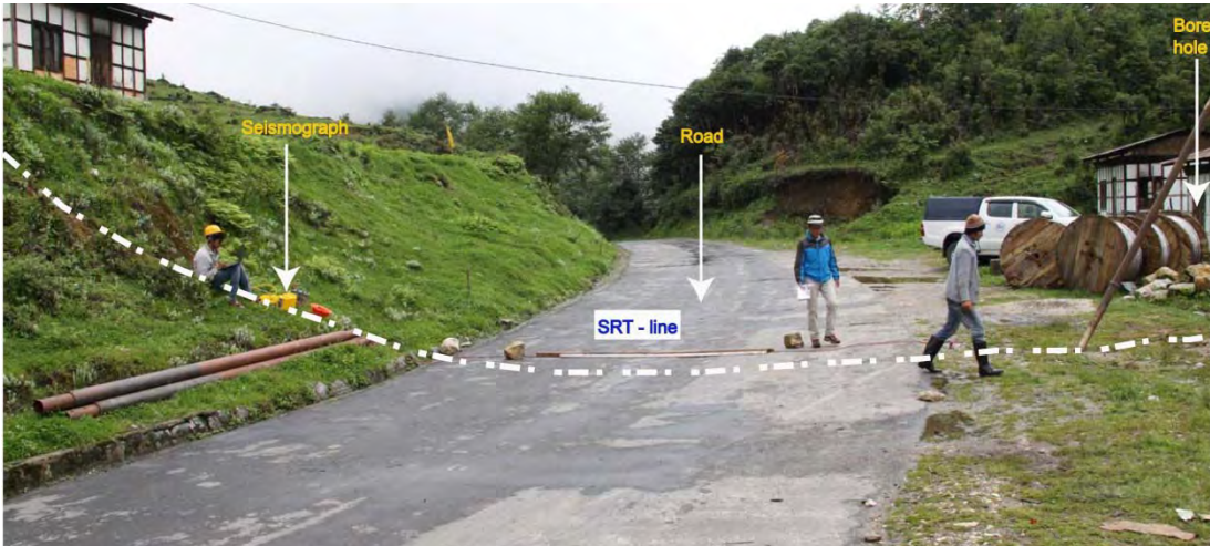
Figure 15: Photograph showing data acquisition along SRT line (white dashed line)
